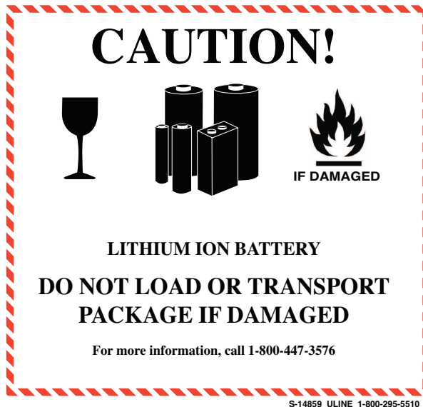
Figure 2-4. Battery handling label.
