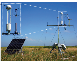
Solar-powered station above measures fluxes of CH 4 , CO 2 and H 2 O, and transmits data wirelessly to closest wired location
