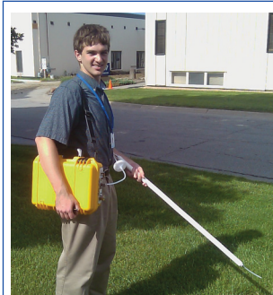
Figure 1. One of the authors with the LI-8100A configured for ground level CO 2 concentration (GLCC) measurement.
