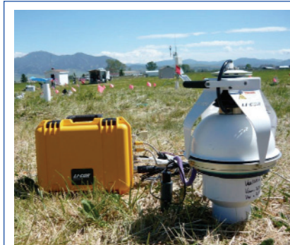
Figure 4. The LI-8100A configured for accumulation chamber measurements at the ZERT site.
