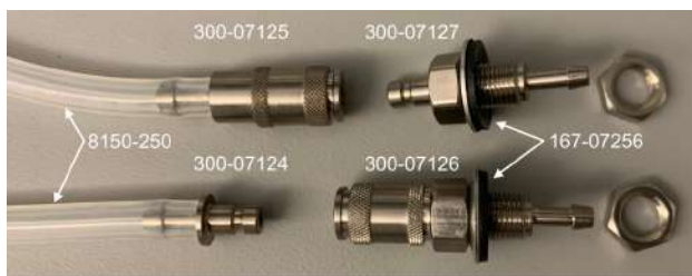
Figure D-4. Pneumatic fittings and tubing are used for flask measurements.
