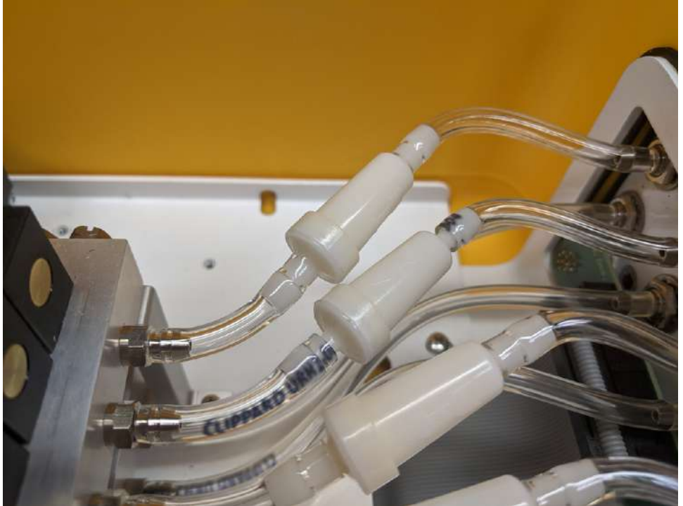
Figure 7-5. Route the tubing to the hose barb at the air inlet, trim the hose, and connect.
