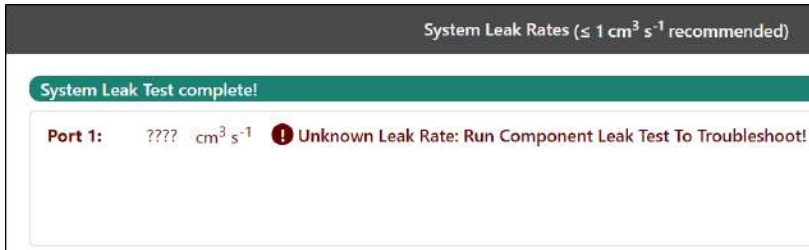
Figure 7-11. Leak test results indicating a high leak rate on port 1.
