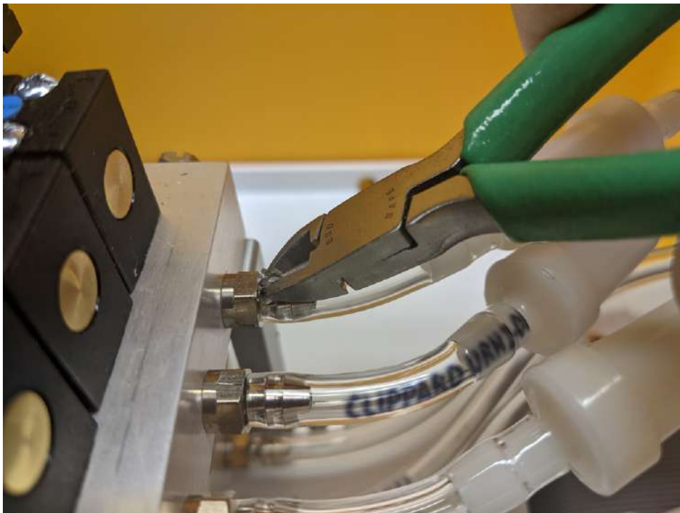
Figure 7-2. Cut a small, wedge-shaped section out of the tubing behind the hose barb.
