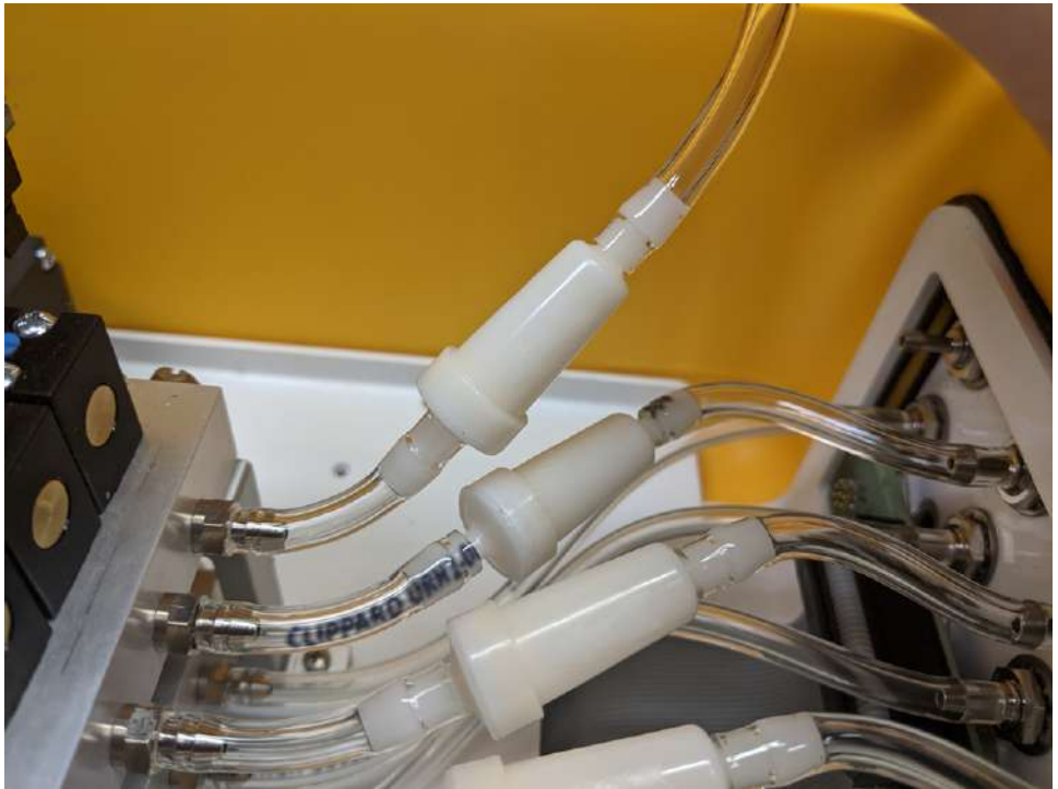
Figure 7-4. Attach the tubing to the hose barb on the valve manifold with the wide end of the filter toward the valve manifold.
