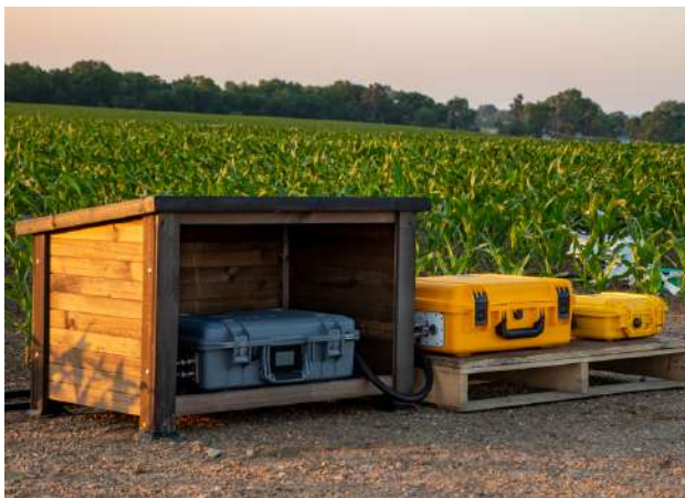
Figure 2-1. An example long-term system setup with an LI-78xx Trace Gas Analyzer, LI-8250 Multiplexer, and LI-870 CO 2 /H 2 O Analyzer.
