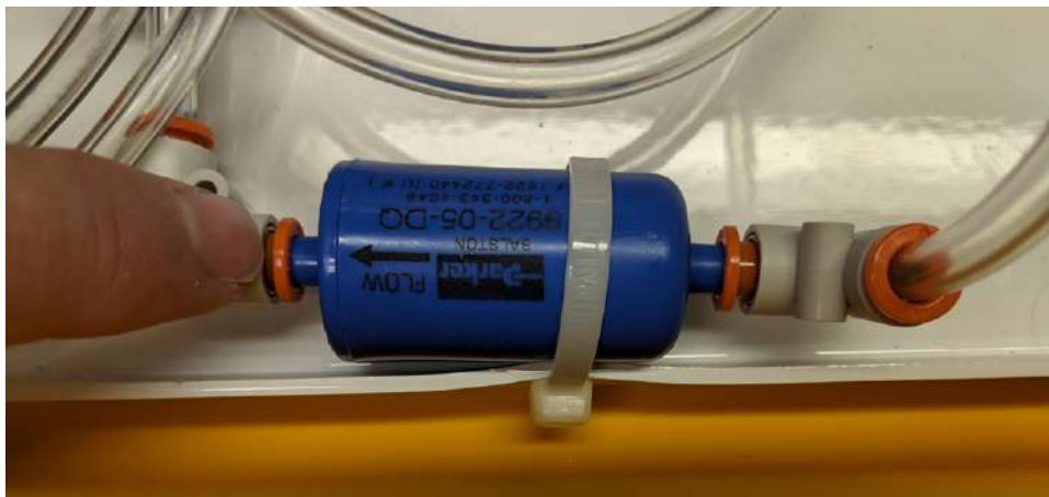
Figure 7-7. Press in on the orange collets to remove the quick-connect fittings and slide the old filter out.
