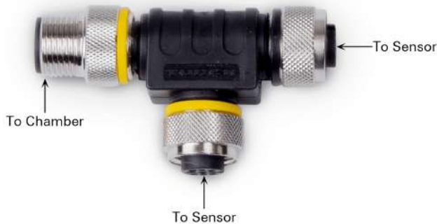
Figure 4-7. One end of the sensor T-split fitting connects to the chamber and the other two fittings are available to connect to a sensor.
