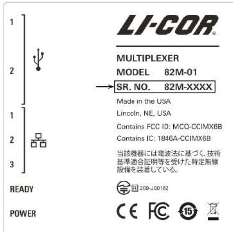
Figure 2-4. The serial number can be found on the interior label of the multiplexer.
