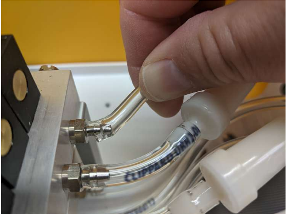
Figure 7-3. Remove the tubing from the hose barb by pulling firmly to the side (perpendicular to the fitting).
