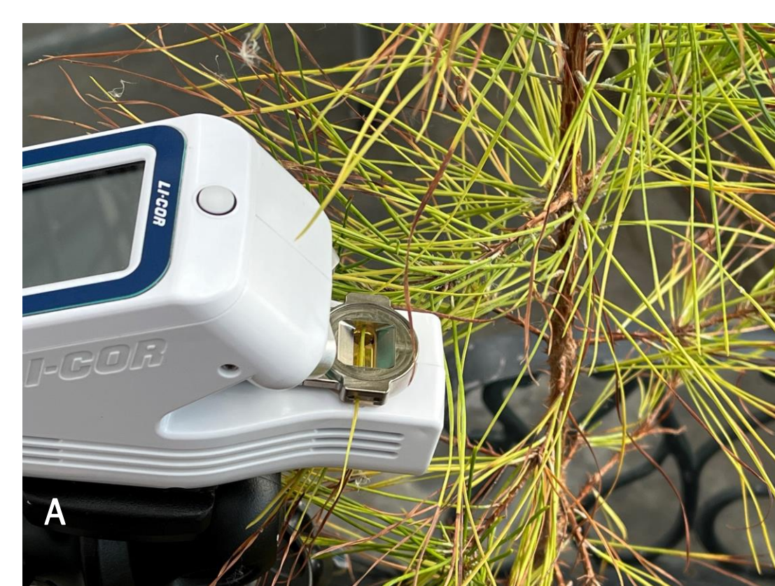
Figure 1: LI-600N Design. (A) LI-600N clamped on a loblolly pine ( Pinus taeda ) needle. (B) LI-600N flow path design.
