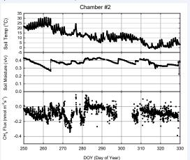
**Example of time serial CH<sub>4</sub> concentration:** With a LI-8100-104 chamber (chamber volume of 4013 cm<sup>3</sup> and soil area of 318 cm<sup>2</sup>), linear regression coefficients were normally higher than 0.9 when the CH<sub>4</sub> flux was higher than 0.1 nmol m<sup>-2</sup>s<sup>-1</sup>. see the two examples below.
