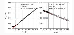
Based on our seasonal longterm methane flux data, we feel confident that this configuration of a closed chamber system can resolve a minimum flux as low as 0.05 nmol m<sup>-2</sup>s<sup>-1</sup>. See an example to the right. Over the two minutes observation, chamber CH<sub>4</sub> concentration decreased by approximately 0.79 ppb (0.0066X120=0.792 ppb).
