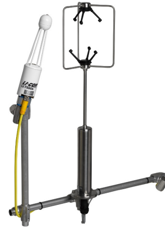
Figure 1. LI-7500A Open Path CO 2 /H 2 O Analyzer and Gill WindMaster sonic anemometer in a typical evapotranspiration setup.
