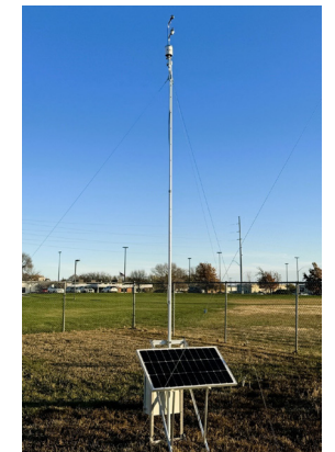
Figure 6: LI-720 sensor deployed on a Carbon-Node
