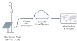
Figure 7: Cloud-integrated LI-710/LI-720 system architecture
